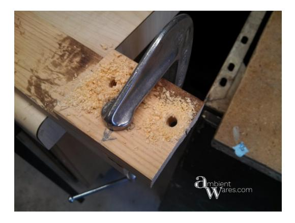
Now that the jig is done, I placed it on top of the plant stand. I slid the drill bit into the jig leaving  $\frac{1}{2}$ " of the bit exposed. Then I taped the drill bit which marks when to stop.
